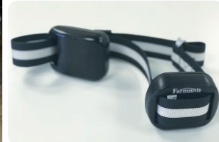
Inputting information using a dedicated smartphone app makes cattle management easy. Using collar-shaped sensors, the farmer can detect changes in health condition to improve the accuracy in capturing each cow's estrus.
