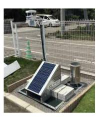
Example installation: POTEKA can accurately forecast wind direction and speed 36 hours in advance to avoid problems with neighboring areas when spraying agricultural chemicals. It can also identifify optimal harvest period by collecting and analyzing data such as accumulated temperature and precipitation.
