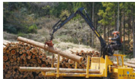
Loading logs with a forwarder
