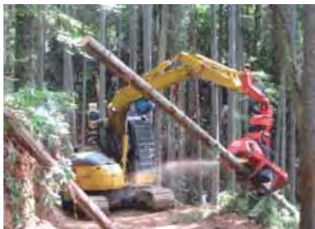
Processing trees into logs with a harvester
