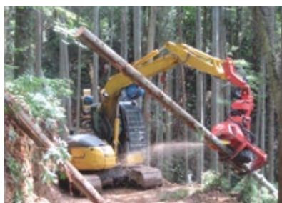
Processing trees into logs with a harvester
