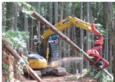
Processing trees into logs with a harvester
